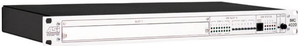
The IMC provides 3 user-configurable RS-232 Serial Ports, and a separate maintenance port. These ports are typically used to interface to serially controlled devices such as Laser Disk Players, CD Players, Video Switchers, Lighting Control Boards, and Programmable Logic Controllers. One Port can optionally be configured to use the 3 pin Mini XLR Jack to transmit DMX-512 for control of Dimmers, Moving Lights, and other DMX-512 controlled devices.
